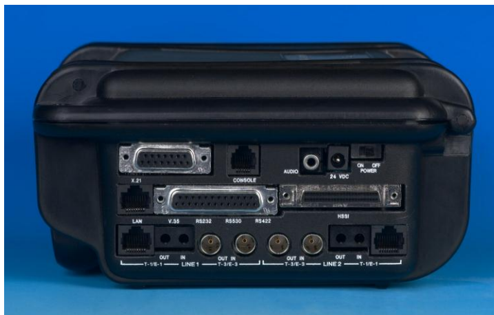
The WAN Tester III is supplied complete with all the interfaces pictured above.
