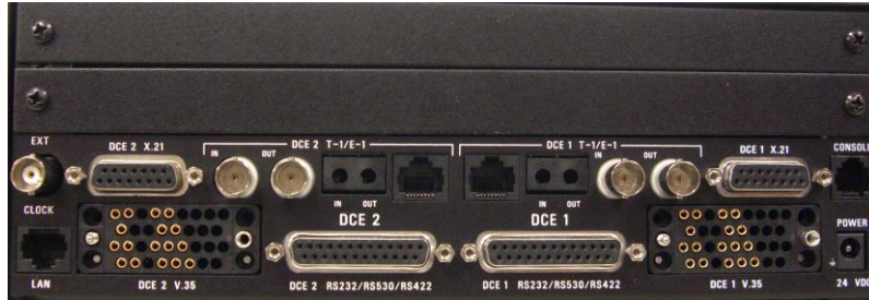
Rear Panel of DLS II showing all standard interfaces and two available option slots.
